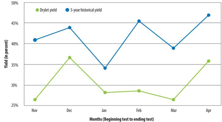
**Figure 2.** 5-year historical yield at 15,000-m<sup>3</sup>/day wastewater treatment plant compared against Drylet testing period yield for each month (lower yield indicates less dry solids produced each month)
