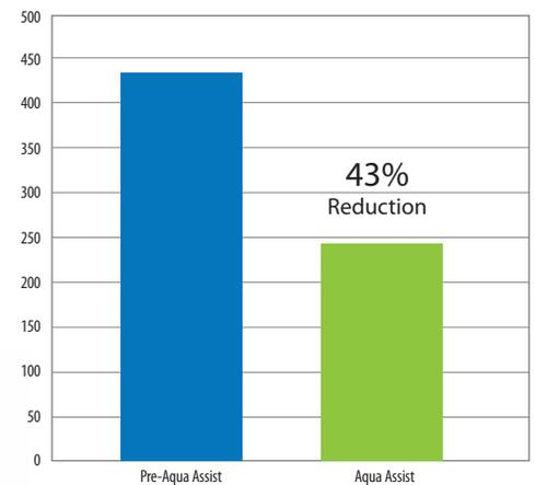
**Figure 3.** 19,000-m<sup>3</sup>/day wastewater treatment plant, average daily waste activated sludge rate (m<sup>3</sup>/day)
